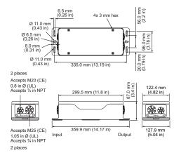
PDS-80 CA 24V, Four-Wire Terminal, 4A 24V, IP66, UL, for Flex Compact and Flex Micro, eW Specification Sheet
