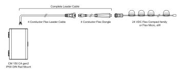
\*A Flex Dongle and 4 conductor Leader Cable is required to create a complete Flex Leader Cable..
