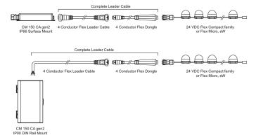
\*A Flex Dongle and 4 conductor Leader Cable is required to create a complete Flex Leader Cable.
